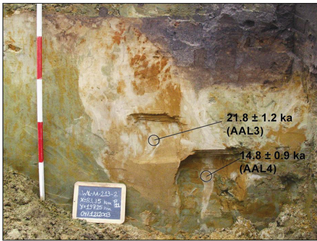
Figure 2. Vertical cross-section of a complex wedge comprising a relict sand wedge (AAL4) which dissects an older composite-wedge pseudomorph (AAL3), Low-Belgium. Numbers refer to the OSL ages (Buylaert et al., accepted).
