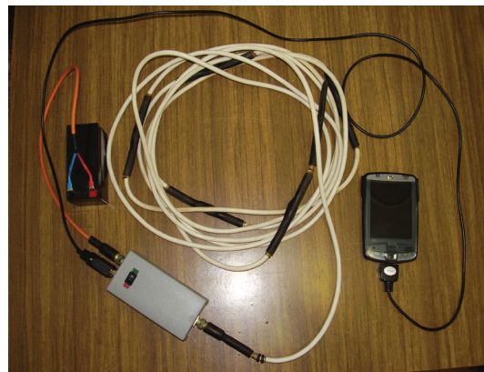
Figure 2. The Thermoscan temperature monitoring system.
