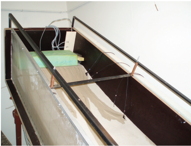
Figure 5. Close-up of the apparatus used in the physical modeling of debris flows.
