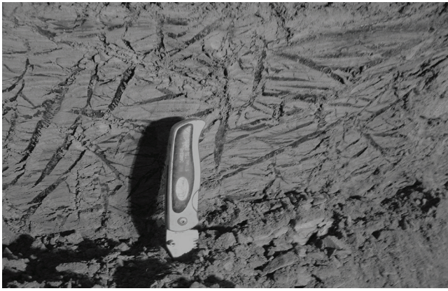
Figure 3. Typical reticulate-chaotic cryostructure with multi-directional interconnected ice veins and ice lenses. The handle of the knife is about 6 cm long.
