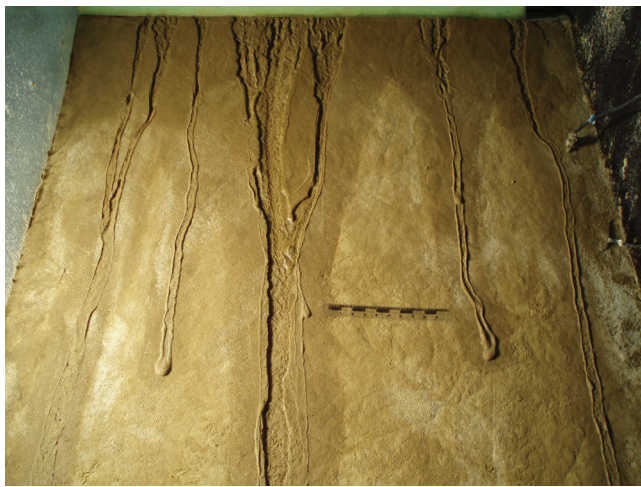
Figure 8. Narrow gullies with lateral levees and relatively small terminal lobes. The morphological characteristics of these gullies on sand are similar to those found on Mars in the Russell Crater. On the top: sinuous channels on the rim crest (like those observed on Mars). In the middle: connections between gullies and variation of their growth by successive wave of debris due to several pulses of water from the rim crest. The analogy with Figures 1 and 2 is striking.
