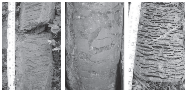
Figure 2. Some types of cryogenetic textures of transitional layer.
