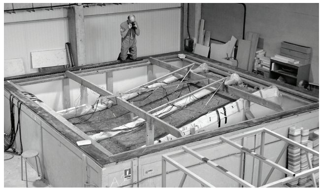
Figure 1. Two parallel slope models, far side, two-sided freezing model, near side, one-sided freezing model. Cross beams support pairs of LVDTs which form fixed base triangles, the apex of which is attached to a Perspex footplate embedded in the soil surface.
