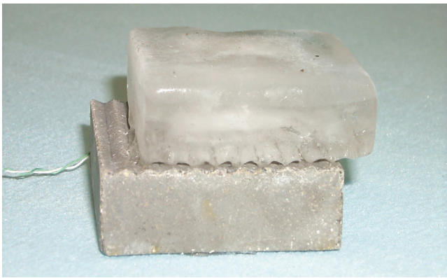
Figure 3. Concrete-ice sample after a constant strain test with normal stress = 207 kPa.
