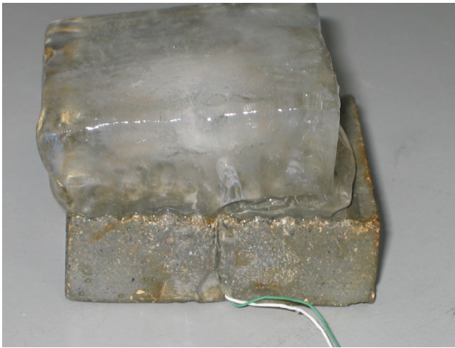
Figure 12. Shear deformation of a concrete-ice sample after a constant strain test with normal stress = 490 kPa.
