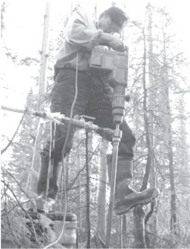
Figure 4. Electric percussion drill with water swivel. This hammer drill has 14A/120V power with 120–250 RPM rotation with impact (energy: 13.3 ft/lb)
