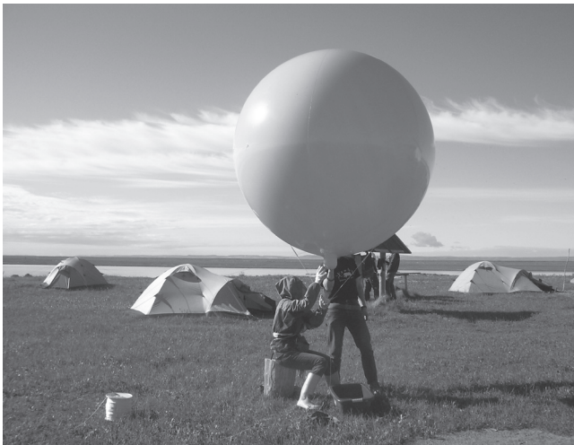
Figure 4. Tethered balloon, filled with helium, diameter 2–3 m.
