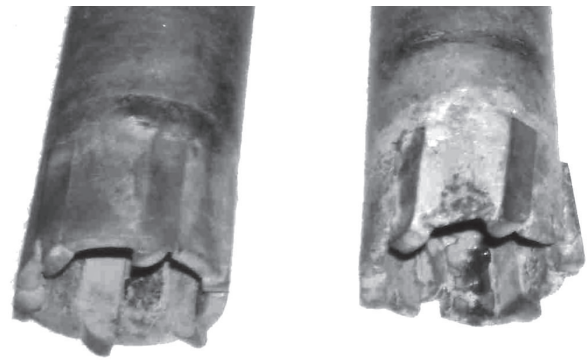
Figure 6. 30 mm diameter core bit for gravel (negative rake angle) (on left) and for silt (positive rake angle) (on right).
