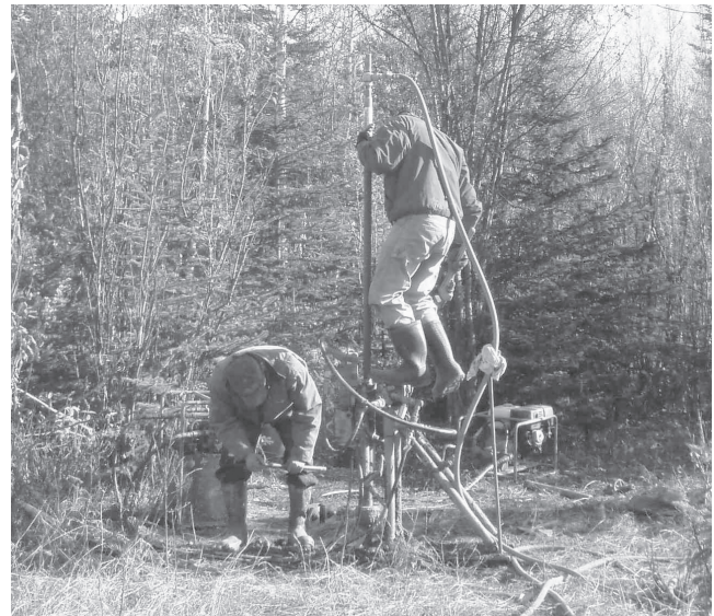
Figure 3. Portable hydraulic spindle (rotary) drill with air swivel. This is lightweight unit compared with track rig machine, but it is still heavy (more than 100 kg) to carry around.
