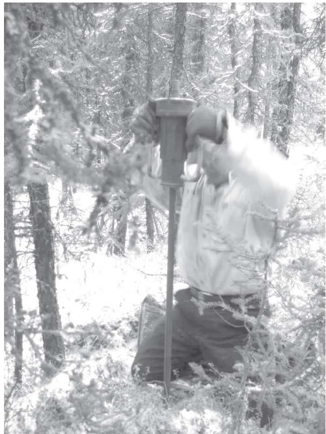
Figure 10. Human-powered traditional percussion system using steel rod.
