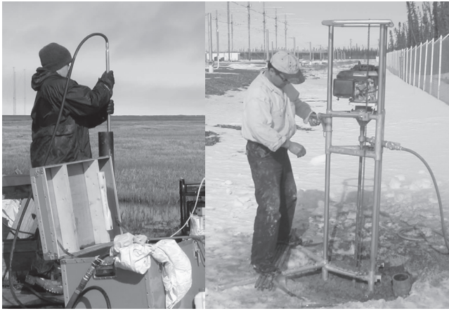
Figure 1. Hot water jet system employed for old borehole (left) and prototype lightweight compact disassembled rotary drill with air swivel (right).
