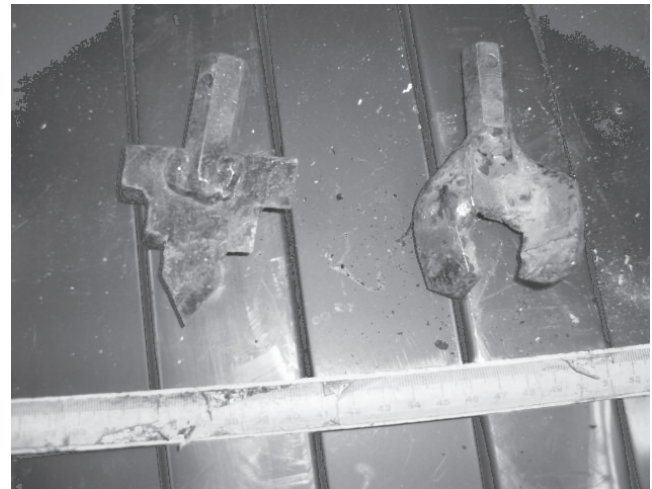
Figure 7. Fifty mm-wide auger bit for multi-grained (no rake angle [left]) and for silt (positive rake angle [right]).
